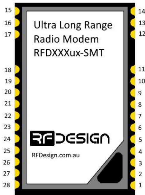
Figure 16: ux-SMT modem pinout
