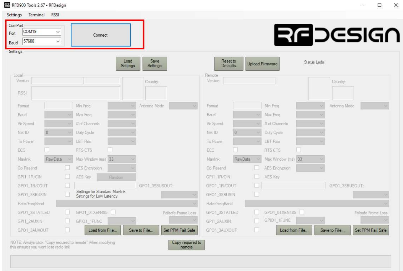
Figure 11: RFD Tools COM port connection
